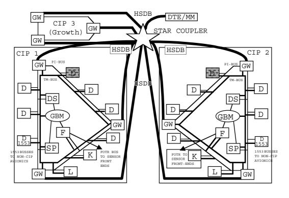
D = DATA PROCESSOR ELEMENT DS = DATA PROCESSOR/SERVER K = KOV-5 L = LLSP SP = SIGNAL PROCESSOR F = FNIU GW = GATEWAY
