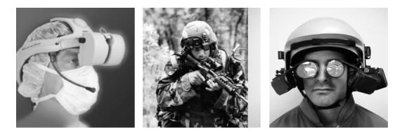
**FIGURE 5.1** Three different applications for HMDs: the CardioView<sup>®</sup> for minimally invasive cardiac surgery (photo courtesy of Vista Medical Technologies, Inc.), a prototype of the U.S. Army Land Warrior HMD (photo courtesy of Program Manager, Soldier, U.S. Army), and the SIM EYE XL100 for aviation training (photo courtesy of Kaiser Electro-Optics).
