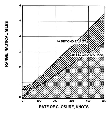
FIGURE 18.5 TA/RA Tau values for sensitivity level 5.
