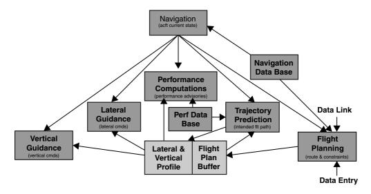
FIGURE 15.2 Flight management functional block diagram.
