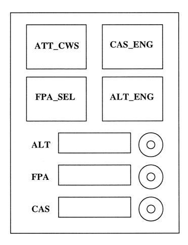
FIGURE 21.2 Mode-control panel.
