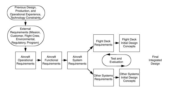
FIGURE 9.1 Simplified representation of the flight deck design process (from NASA TM 109171).
