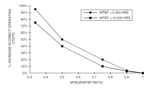
FIGURE 25.1 MTBUR/MTBF ratio impact of operating costs.
