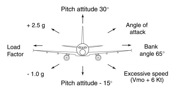
FIGURE 12.6 A320 flight envelope protections.
