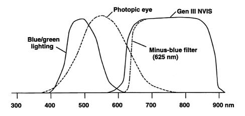
FIGURE 7.8 Typical Class A blue-green lighting and 625-nm minus-blue coating on NVIS.
