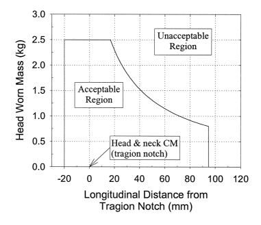
**FIGURE 5.10** The USAARL weight and horizontal center of gravity curve with the area under the curve considered acceptable for fatigue in helicopter environments. (Data curve courtesy of U.S. Army Aeromedical Research Labs, used with permission.)
