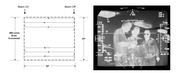
FIGURE 4.13 Bi-directional scan-converted raster image.
