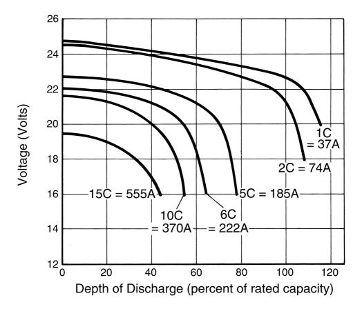
FIGURE 10.2 Discharge curves at 25°C for a 24 V/37 Ah SLA aircraft battary.
