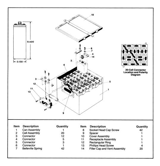
FIGURE 10.5 Assembly drawing of a nickel-cadmium aircraft battery.
