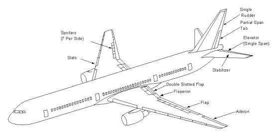
FIGURE 11.1 The Primary Flight Control System on the Boeing 777 is comprised of the outboard ailerons, flaperons, elevator, rudder, horizontal stabilizer, and the spoiler/speedbrakes.
