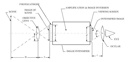
FIGURE 7.3 Typical NVIS image intensifier tube and optics.
