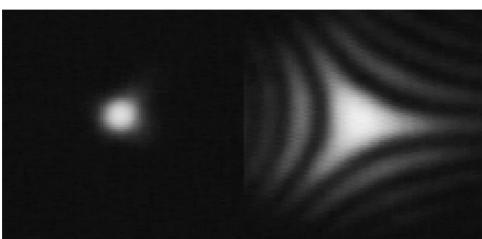
**FIGURE 6.4** The effect of improved mirror design is visible in these spot (pixel) images, normalized for size but not for intensity, for scanned spots at  $\sim \lambda/4$  P-P mechanical mirror deformation (left image), and  $\sim 2\lambda$  P-P mechanical mirror deformation (right image).
