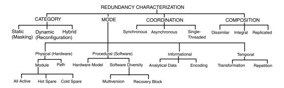
FIGURE 28.5 Redundancy classification.
