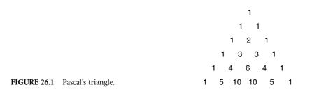
As an example of the use of arrays suppose we wish to compute the successive rows of Pascal's triangle. This is usually represented as shown in Figure 26.1. The reader will recall that the rows are the coefficients in the expansion of  $(1 + x)^n$  and that a neat way of computing the values is to note that each one is the sum of the two diagonal neighbors in the row above.
