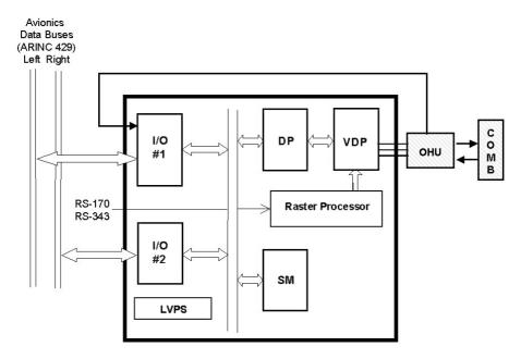
FIGURE 4.11 High integrity HUD computer architecture.
