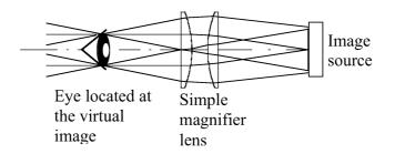
FIGURE 5.6 Diagram of a simple magnifier, or non-pupil-forming lens.
