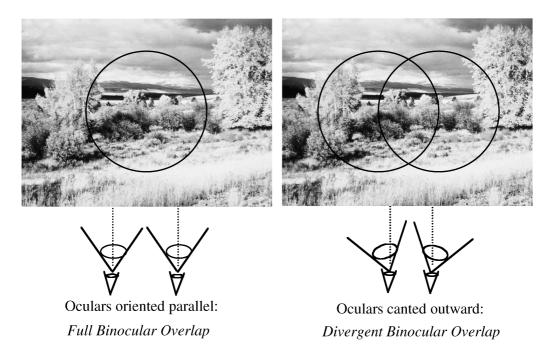
**FIGURE 5.14** Comparison of a full binocular overlap and divergent partial binocular overlap. Note the increase in viewable imagery in the horizontal direction with the divergent overlap.
