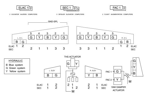
FIGURE 12.3 A320/A321 flight control system architecture.
