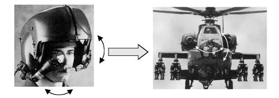
**FIGURE 5.11** The linkage between the IHADSS helmet-mounted display and the Pilot's Night Vision System in the AH-64 Apache helicopter. The PNVS is slaved to the pilot's head line of sight. As he turns his head, the PNVS turns to point in the same direction.
