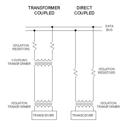
FIGURE 1.2 Terminal connection methods.
