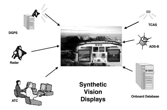
FIGURE 16.1 Possible synthetic vision system.
