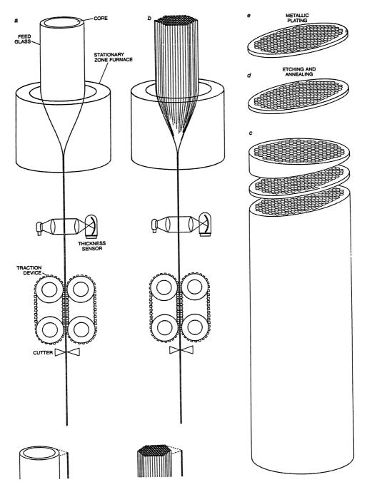
**FIGURE 7.2** Double glass draw for MCP manufacture<sup>1</sup>.
