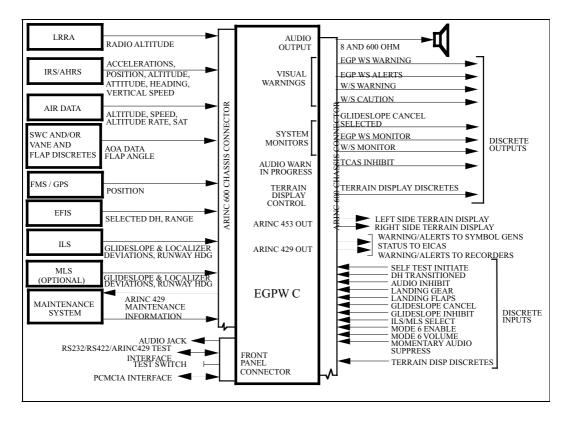
FIGURE 17.1 Typical air transport EGPWS installation.
