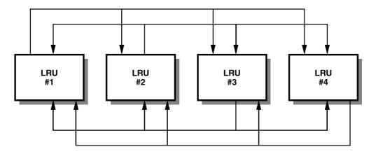
FIGURE 3.2 Bidirectional CSDB communication.
