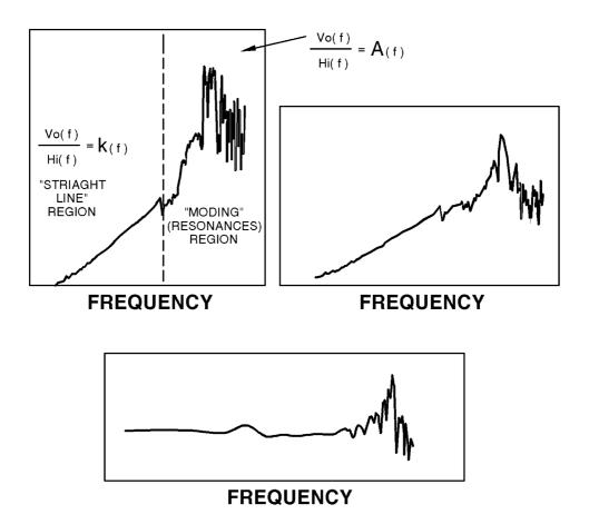
FIGURE 25.8 Frequency domain representation of EME energy attenuation/coupling transfer functions.
