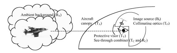
FIGURE 5.15 Contributions for determining image source luminance requirements for an HMD in an aircraft cockpit.
