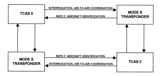
FIGURE 18.2 Interrogation/Reply between TCAS systems.
