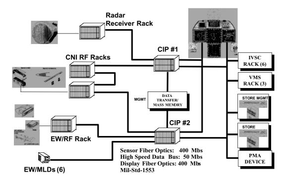
FIGURE 32.3 Avionics system architecture.
