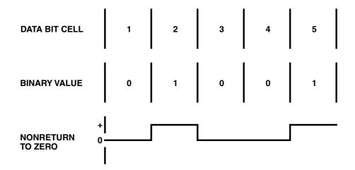
FIGURE 3.4 Non-Return to Zero data example.
