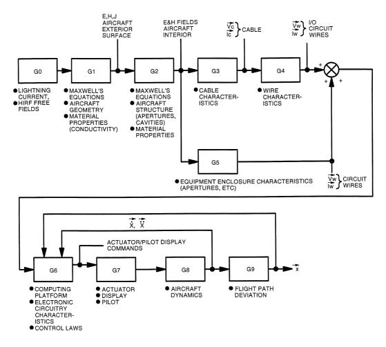
FIGURE 25.4 EME propagation process transfer function perspective.
