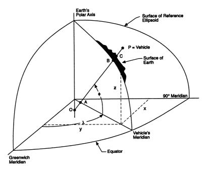
**FIGURE 13.1** Latitude–longitude–altitude and x,y,z, coordinate frames.  $\phi$  = geodetic latitude;  $\overrightarrow{OP}$  is normal to the ellipsoid at B;  $\lambda$  = geodetic longitude;  $h = \overrightarrow{BP}$  = altitude above the reference ellipsoid = altitude above mean sea level.
