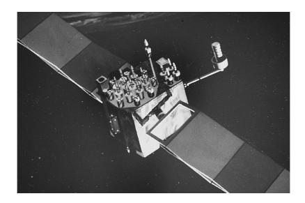
**FIGURE 13.5** Global positioning satellite, Block 2F. L-band phased array and S-band control antennas are visible Steerable solar panels power the Spacecraft. Orbit altitude is 10,900 nmi at a 12-hour period. (Courtesy of Rockwell.)
