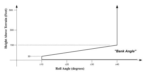
FIGURE 17.9 EGPWS Mode 6 overbank (excessive roll) alert.
