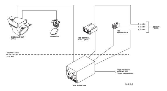
FIGURE 4.8 HUD interconnect diagram (RCFD HGS-4000).
