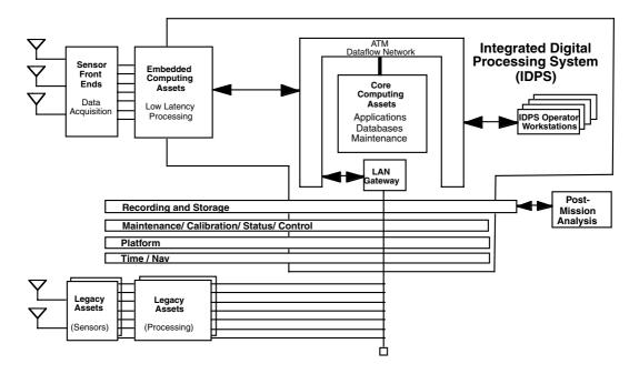
FIGURE 20.3 A generalized integrated avionics architecture.
