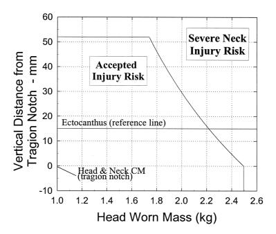
**FIGURE 5.9** The USAARL weight and vertical center of gravity curve. The area under the curve is considered crash safe in helicopter environments. (Data curve courtesy of U.S. Army Aeromedical Research Labs, used with permission.)
