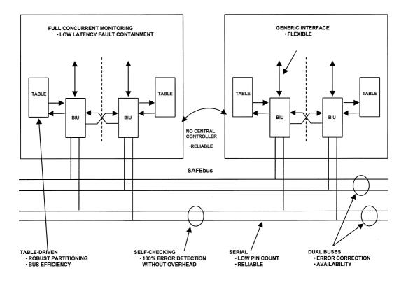
FIGURE 29.5 SAFE bus<sup>TM</sup> dual serial buses.
