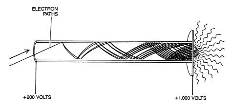
**FIGURE 7.1** Electron amplification in a microchannel.<sup>1</sup> © 2001 by CRC Press LLC
