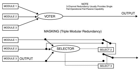
RECONFIGURATION (Triplex Redundancy)
