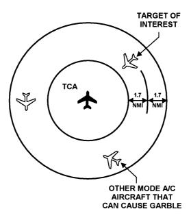
FIGURE 18.3 Synchronous garble area.
