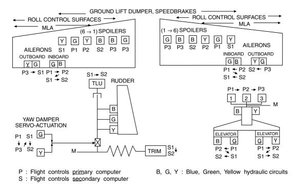
FIGURE 12.4 A330/A340 flight control system architecture.
