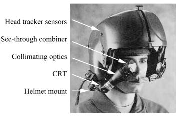
FIGURE 5.3 The Honeywell IHADSS is a monocular, monochrome, CRT-based, head-tracked, see-through helmet-mounted display used on the U.S. Army AH-64 Apache helicopter. (Photo courtesy of Honeywell Electronics, used with permission.)
