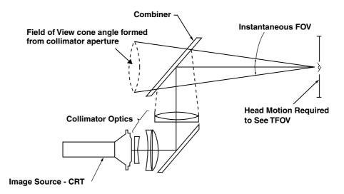
FIGURE 4.4 Refractive optical systems.
