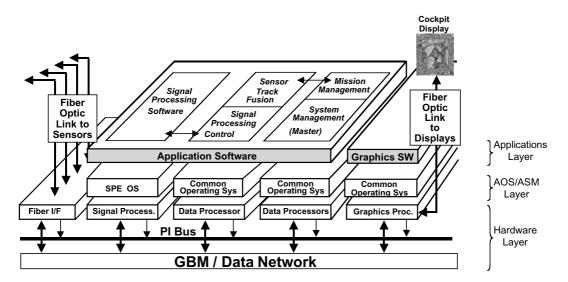
FIGURE 32.5 CIP processing architecture.
