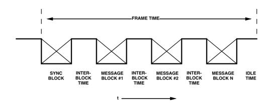
FIGURE 3.3 CSDB data frame structure.
