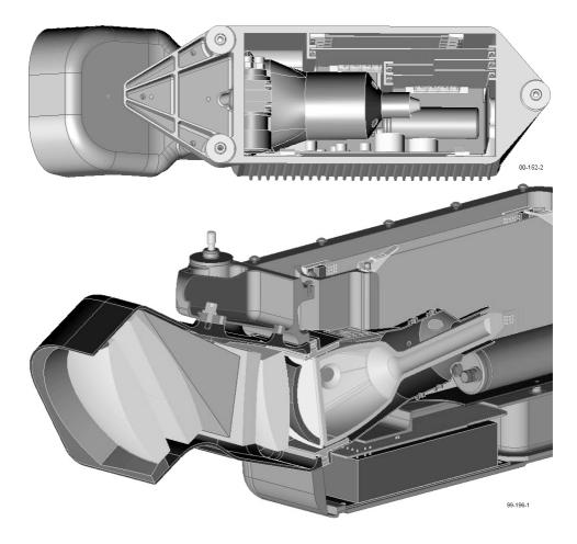
FIGURE 4.9 HUD overhead unit chassis (WFOV reflective optics).
