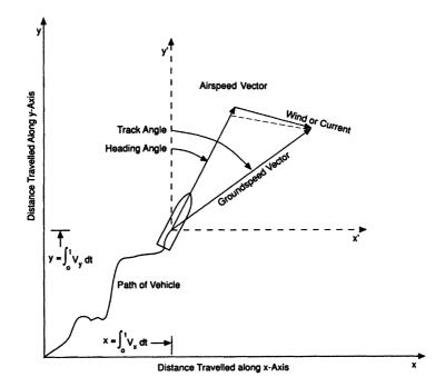
FIGURE 13.2 Geometry of dead reckoning.
