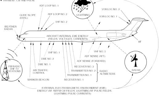
FIGURE 25.2 External EME (HIRF, lightning) interaction.
