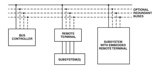
FIGURE 1.3 Simple multiplex architecture.
