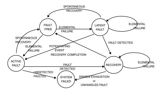
FIGURE 28.4 Hardware states (with corrective action).
