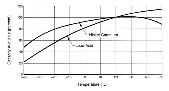
FIGURE 10.4 Capacity vs. temperature for aircraft batteries at the C-rate.
