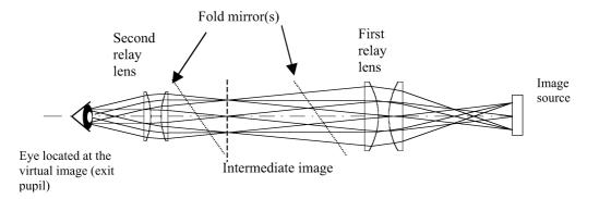
FIGURE 5.7 A pupil-forming optical design is similar to a compound microscope, binoculars, or a periscope.
