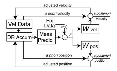
FIGURE 14.2 Position and velocity estimation.
