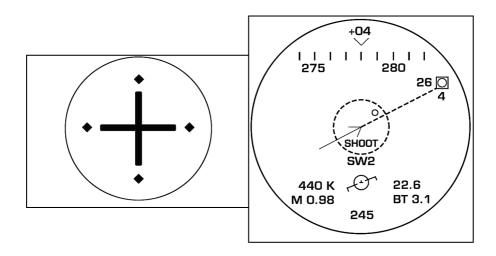
**FIGURE 5.5** Comparison of early HMD reticle imagery (left) with a more capable symbology set (right) to be used with the HMDs such as the JHMCS.
