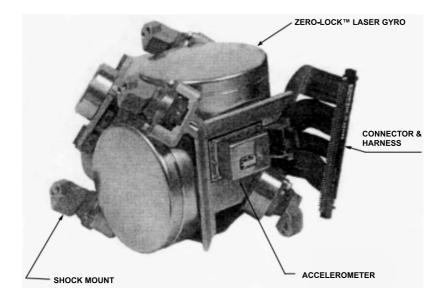
**FIGURE 13.4** Inertial reference unit. Two laser gyroscopes (flat discs), an accelerometer, an electrical connector, and four shock mounts are visible. This unit is used in Airbuses and many military aircraft such as the F-18 and Comanche helicopter. (Courtesy of Litton Guidance and Control Systems.)
