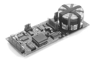
**FIGURE 13.3** Saturated core ("flux-gate') magnetometer, mounted on a "compass engine" board. The two orthogonal sensing coils (visible) and the drive coil, wound on the toroidal core, measure two components of the magnetic field in the plane of the toroid. (Courtesy of KVH Industries, Inc.)
