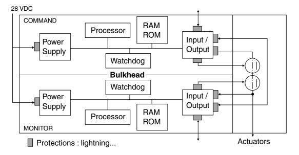
FIGURE 12.5 Command and monitoring computer architecture.
