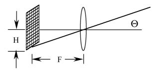
**FIGURE 5.12** The focal length of the collimating lens determines the relationship between H, the size of the image source (or pixel size) and  $\Theta$ , the field of view (or the resolution).
