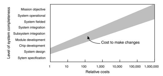
FIGURE 20.1 Relative cost of defect discovery has been shown to increase as a factor of 10 at each successive level of system completeness [Portelli et al., 1989].
