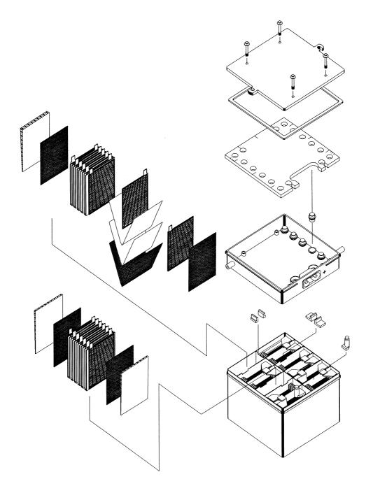
FIGURE 10.1 Assembly drawing of a lead-acid aircraft battery.
