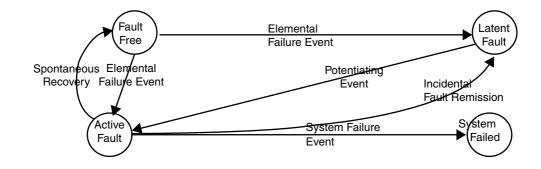
FIGURE 28.2 Hardware states (no corrective action).
