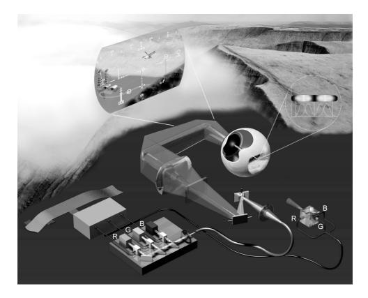
FIGURE 6.1 Functional component diagram of the RSD HMD.
