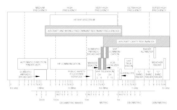
FIGURE 25.3 RF spectrum and associated installation dimensions of interest.
