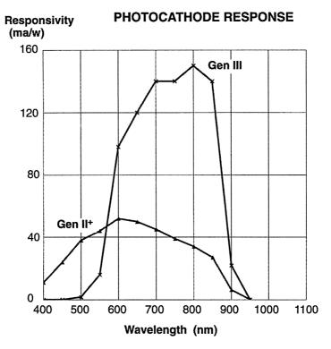
FIGURE 7.4 Photocathode sensitivity.
