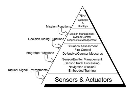
FIGURE 32.2 Avionics functional hierarchy.
