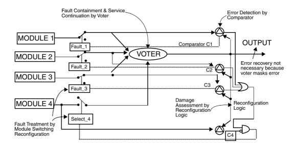
FIGURE 28.7 Hybrid TMR arrangement.
