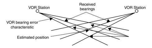
As can be seen from the diagram, the estimated position uncertainty (EPU) is dependent on the error characteristics of the particular navigation system being used as well as the geometric positioning of the navaids themselves. Other navigation sensors such as an inertial reference system have error characteristics that are time-dependent. More information pertaining to EPU and various navigation navaid system error characteristics can be found in RTCA DO-236.
